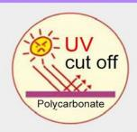
There is a co-extrusion UV coating on the surface which can effectively block up to 98% of UV rays.
